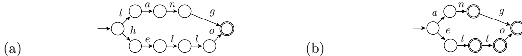
Figure 6: (a) \mathbf{A} , \mathcal{L}(\mathbf{A}) = \{lang, hello\} . (b) \mathbf{A}' = SS^\sharp(\mathbf{A}, [1, 1], [3, +\infty]) , \mathcal{L}(\mathbf{A}') = \{an, ang, el, ell, ello\} .
