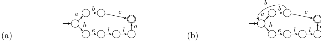
Figure 7: (a) A_1 , \mathcal{L}(A_1) = \{abc, hello\} . (b) A_2 , \mathcal{L}(A_2) = \{abc, hello\} \cup \{(abb)^n c \mid n > 0\} .
